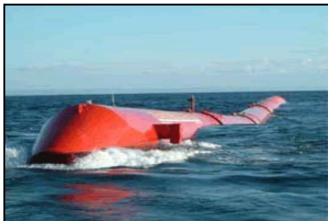
Photo of a Pelamis wave energy converter www.pelamiswave.com/content.php?id=161
